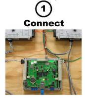
Connect includes: Mounting and wiring the controller and interface panels.
